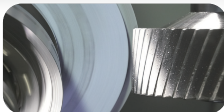
External gear profile grinding
